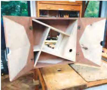
▲ Pic.41 I decided to assemble it, then fitted the back panel and the hanging plates, before moving on to shooting the doors to size. I sanded them followed by the whole cabinet
